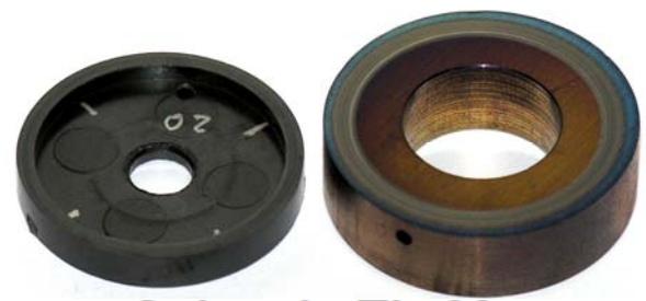
Celazole TL-60 & thrust surface 200 fpm
