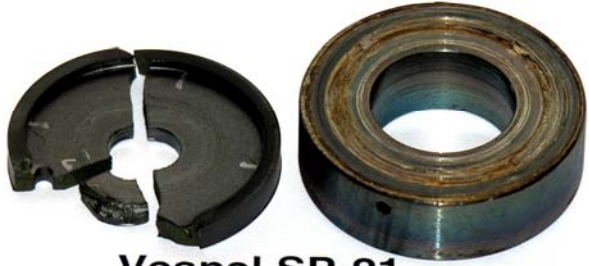
Vespel SP-21 & thrust surface 200 fpm
